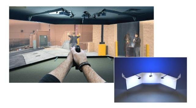
The Ti RECON 180 \* projects up to 33' wide and incorporates our 180 degree mobile screen system. No matter what your training objectives are, your RECON 180 system can accommodate them. The Virtual Marksmanship Mode has up to 12 lanes of fire and with a quick and easy adjustment you can switch to a 180 degree judgment scenario training in a completely immersive environment.
